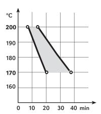
substrate temperature versus curing time
