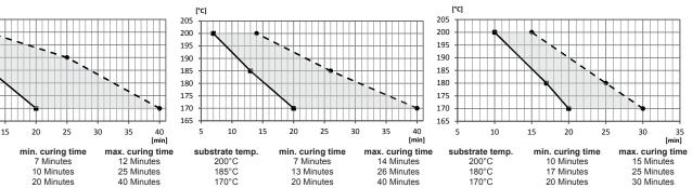
Please observe cure parameters closely since mechanical properties will develop before full cross-linking!
