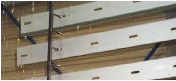
Fig. 1.1.3 Potential transfer of pretreatment media
