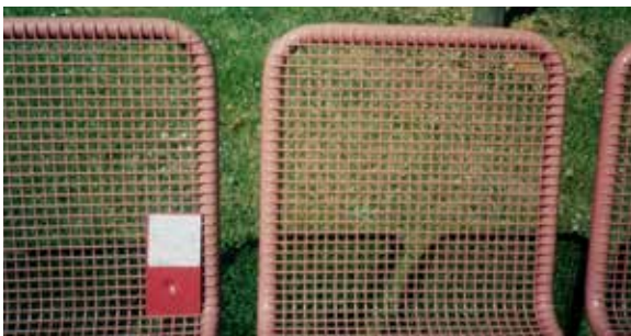
Fig. 5.1.1 Not sufficiently resistant to cleaning agents
