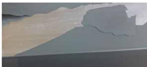
Fig. 1.1.5 Conversion too thick
