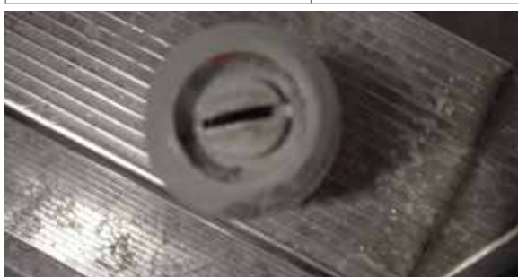
Fig. 2.2.1 Sintering on flat spray nozzle
