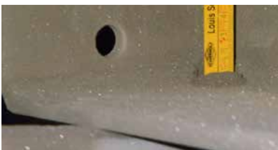
Fig. 2.3.5 Powder layer too thick
