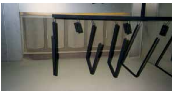
Fig. 3.5.5 Transfer of powder dust - situated too closely together
