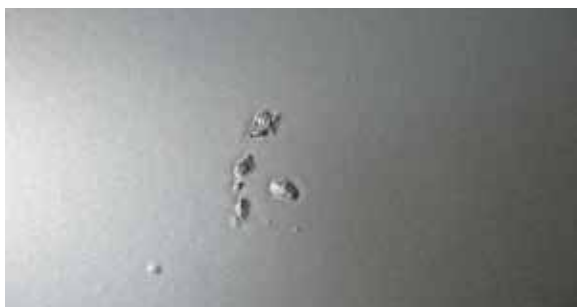
Fig. 3.1.1 Metallic pigment splotches
