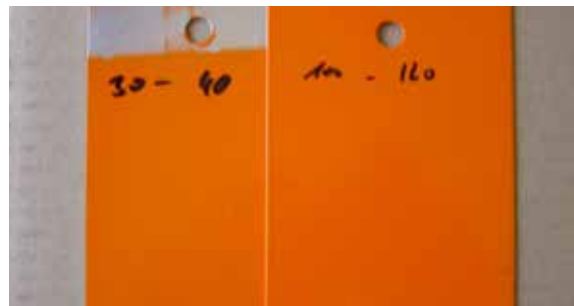
Fig. 4.1.2 Paint films that are too thin and do not cover
