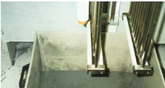
Fig. 2.1.1 Fluidization - powder must flow like water
