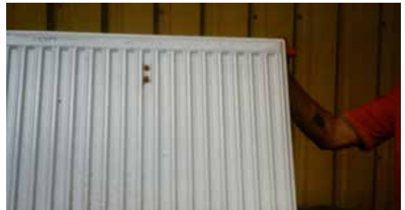
Fig. 5.2.2 Pretreatment unsuitable or insufficient
