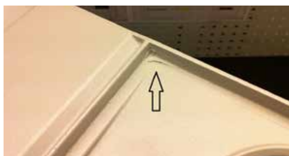
Fig. 3.7.2 Powder-coating accumulation in corners due to powder that trickled off
