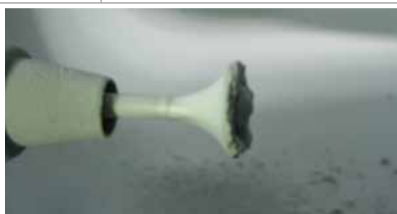
Fig. 2.2.2 Sintering on impact mill
