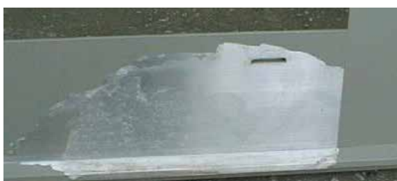
Fig. 1.1.1 Poor (no) chromating
