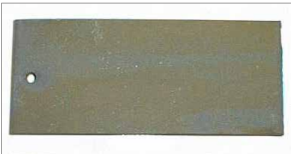
Fig. 1.3.5 Corrosion due to Fe-phosphate coating on sandblasted workpieces
