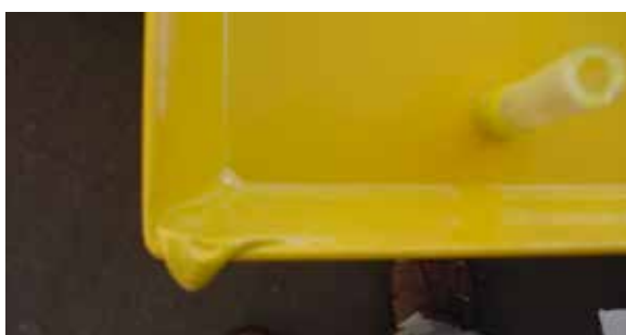
Fig. 3.7.1 Layer thickness too high
