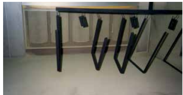
Fig. 6.1.2 Potential transfer of powder from one booth to another – cross contamination
