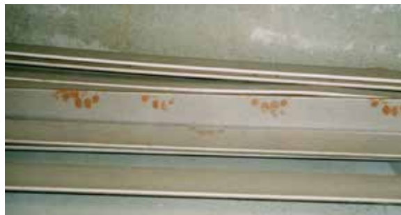
Fig. 3.8.2 Contamination due to hand sweat, hand cream, ...
