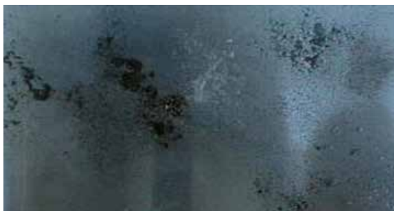
Fig. 1.3.1 Grease residues after pretreatment
