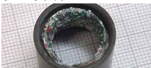
Fig. 2.2.5 Unsuitable hose material
