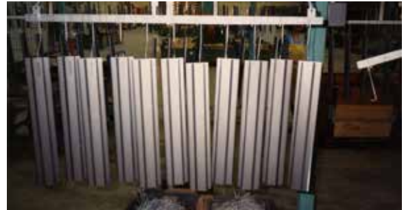
Fig. 2.4.2 Incorrect positioning of workpieces
