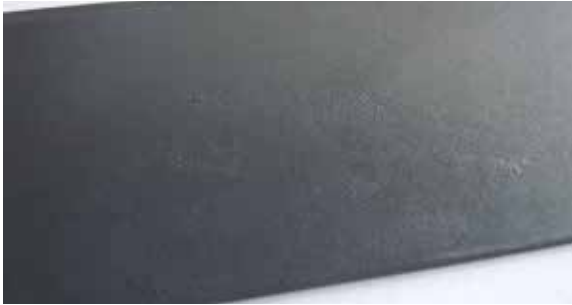
Fig. 3.2.7 Poor rinsing sandblasted, e-coat as base
