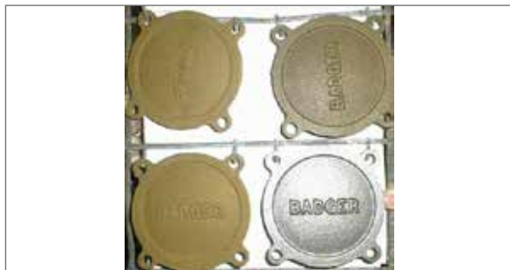
Fig. 1.3.6 Corrosion of sandblasted workpieces after pretreatment
