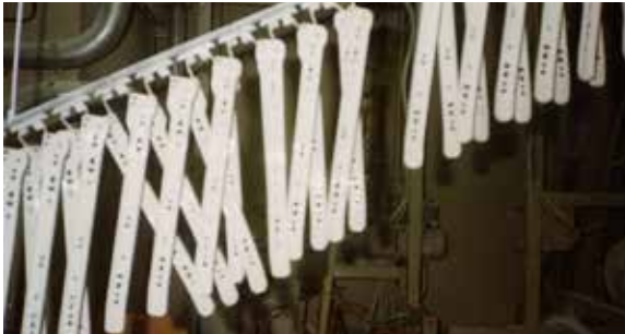
Fig. 2.4.1 Incorrect positioning of workpieces
